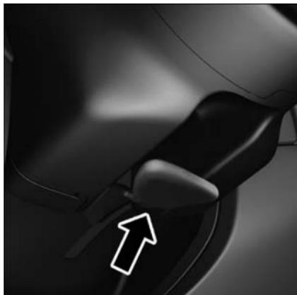
Manual Tilt/Telescoping Steering Column Handle
