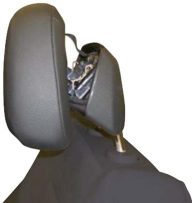
**Active Head Restraint (AHR) Deployed**
