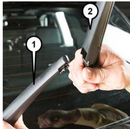
**Wiper Blade Removed From Wiper Arm**
