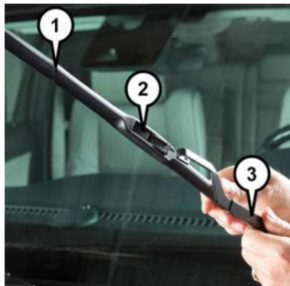
**Wiper Blade Removed From Wiper Arm**
