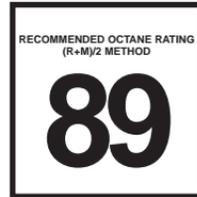
diately. Use of gasoline with an octane number lower than 87 can cause engine failure and may void or not be covered by the New Vehicle Limited Warranty.
