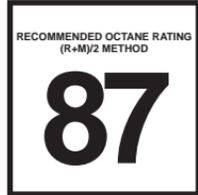
These engines are designed to meet all emissions regulations and provide optimum fuel economy and performance when using high quality unleaded “Regular” gasoline having a
